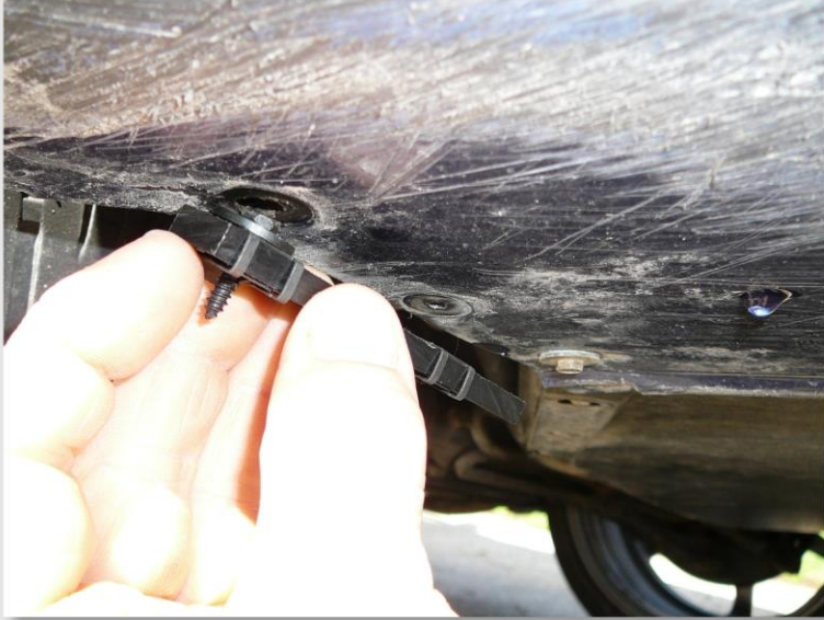
4. Position head of screw in hole and align parallel with fender liner
