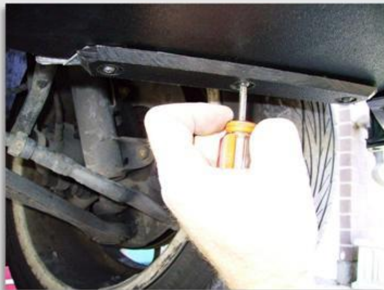
5. Sandwich fender liners between panel & reinforcements
