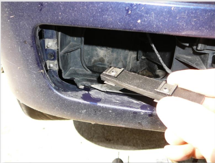
6. Insert reinforcement into fog light hole
