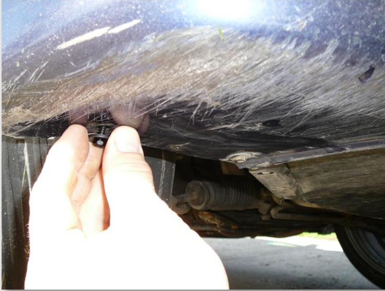
7. Position first screw and thread into outer spring nut
