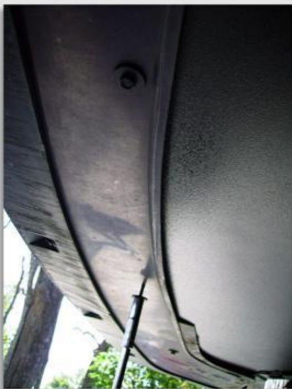
4. Add U-Nuts, place panel on top side of bumper & Insert screws
