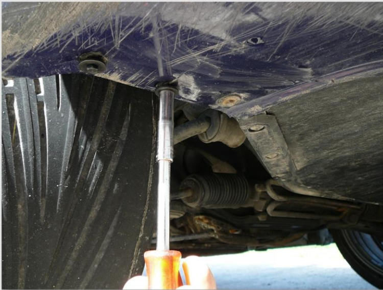
8. Thread second screw through second hole & into the other spring nut
